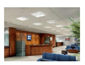
Surface mounting decorative mirror optic luminaire suitable for twin compact fluorescent lamps 18W PL-C.
